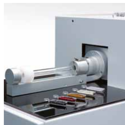
Double furnace technology—determination of the TOC in solids
