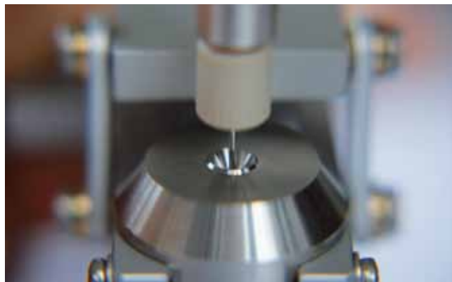
Direct injection: acidifying, purging, injecting
