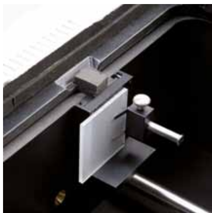
Solid sample holder to determine transmission characteristics
