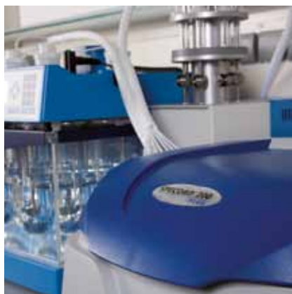
The SPECORD® PLUS Dissolution can be used to examine the release of active ingredients in tablets during the dissolution process.
