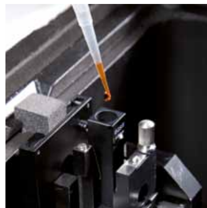
Adjustable cell holder with ultra-micro cell for precise quantitative analysis of extremely small sample volumes
